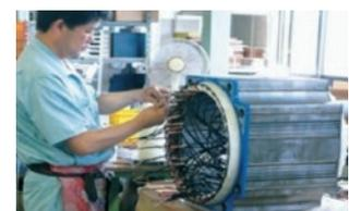
Servomotor electrical works
